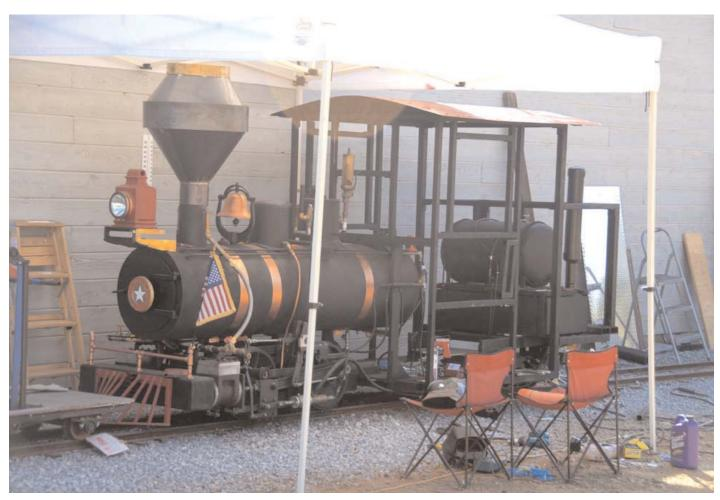
Work is progressing on Doc Hemp's newest locomotive "the Big Brute". Modeled after the Forney locomotives, the engine was built by Harris Locomotive Works. Doc Hemp and Dave Moeller will be finishing up the details. For more information, check out Hemp's website: http://www.dochemp.com/forney.html
