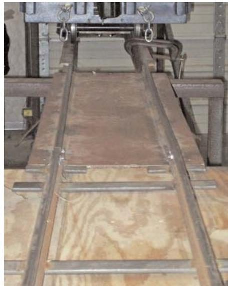
holds the car (or locomotive). There is a hole in both where a bolt is placed, and nut tightened. Now the car (or locomotive) can ride smoothly from truck to car stand and the four foot plate cannot move and does not flex badly under my locomotive, and not at all under my flat cars.
