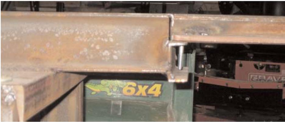
The bolts are ¼ inch diameter and about 2 inches long. There are no nuts. The car stop lifts off when needed. This is not a great system since the car rolls back and forth from end to end. I now use a clamp on the channel iron, clamped right against the wheel as shown below.
