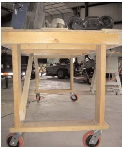
table uses two by four legs with a two by four cross piece that hold three inch casters well. But this table will hold my 300 pound cars, so I used six inch casters. I could have used steel casters that are five inch diameter and two inches wide on the concrete of my barn floor.
