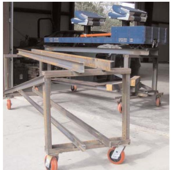
give it better support side to side. A locomotive weighs more than a car, so I felt that it should be wider to be more stable. My loco weighs 1405 pounds, so I am happy to have the wider stand. My flat cars weigh 300 pounds and the 27 inch wide cross pieces are rock solid with this weight or even with one on top and one below.
