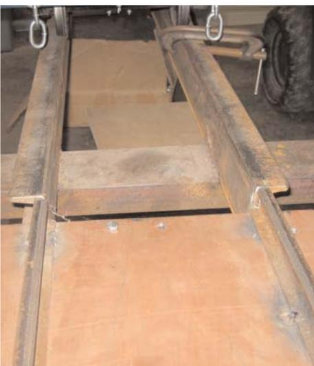
end the four foot plate sits on a piece of channel iron welded to the end of the 3 inch channel iron that
