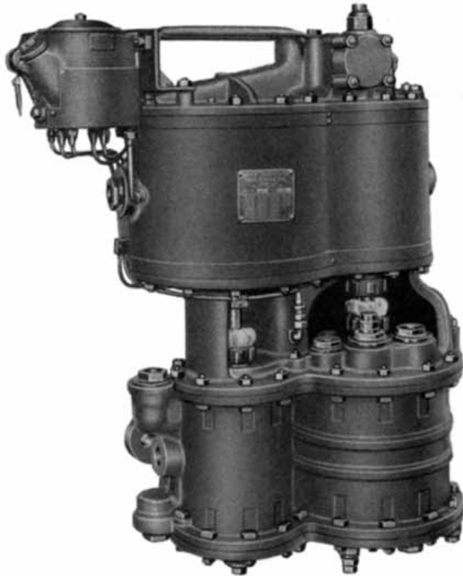
Fig. 20. Front View of the Air Compressor with the "F-1-A" Lubricator
